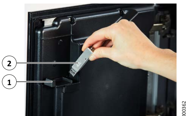
Fig. 30: Inserting the USB stick
