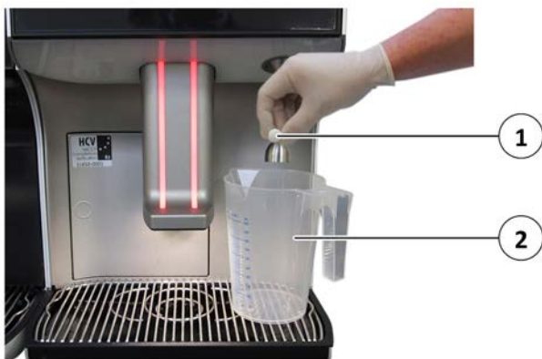
Fig. 42: Preparing the cleaning of the milk system
